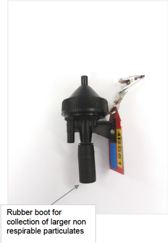
Figure 4. Examples of air samplers used for collecting airborne dust.
